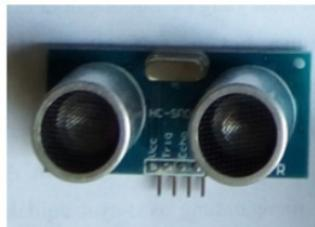
Gambar 3. Sensor ultrasonik HC-SR04
