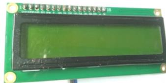
Gambar 5. LCD 16x2
