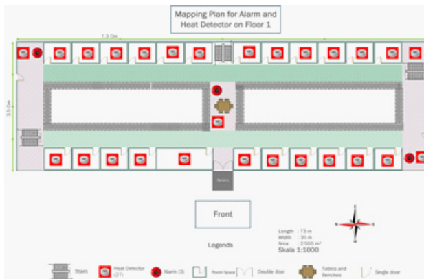
Figure 6. Mapping Recommendation for Dormitory Building on Floor 1 Containing Alarm and Heat Detector Number and Hydrant Requirements after Analysis was Conducted
