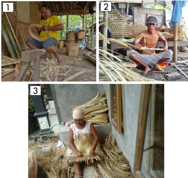
Figure 1. The activity in the woven bamboo industry: (1) Making hard-shaped product frame, (2) Making sharpened and Mashed-bamboo sheets, (3) Waving bamboo sheets
