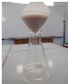
Filter the sediment with filter paper
